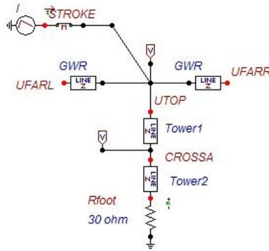
Figure 4: ATP Draw Circuit Diagram
