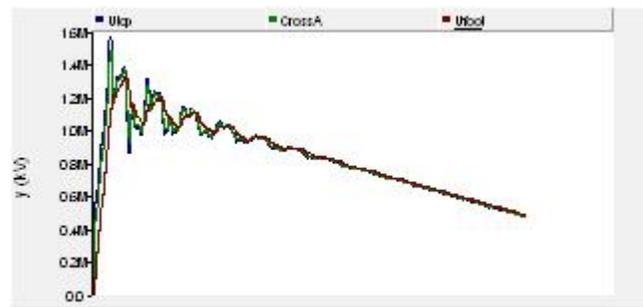
Figure 3: Voltages at tower top, cross arm and footing resistance in PSCAD
