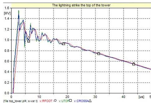
Figure 5: Voltages at tower top, cross arm and footing resistance in ATP
