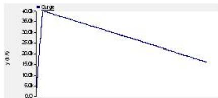
Figure 1: Lightning current in PSCAD
