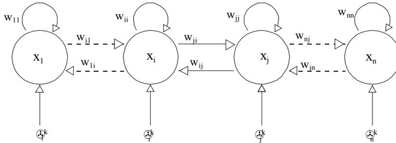
Fig. 1. Single layer recurrent neural network
