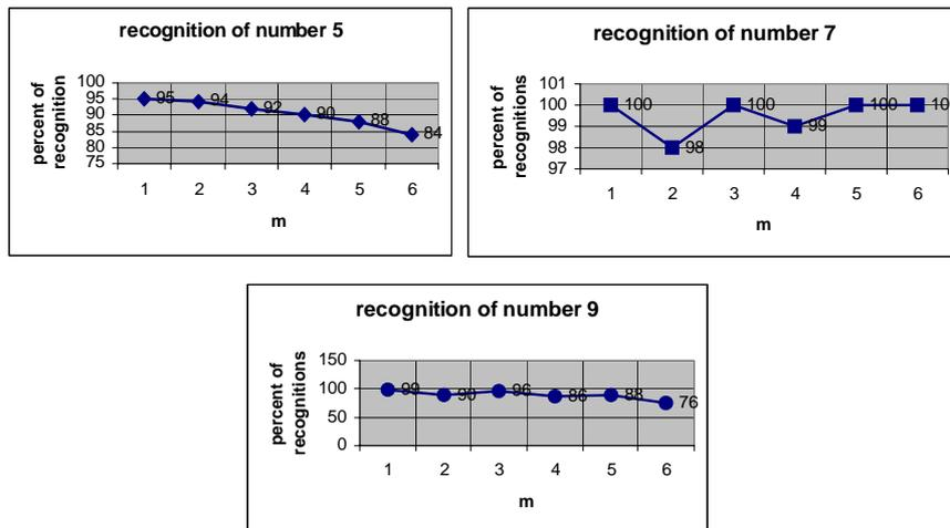
Fig. 2. Recognition of some noisy prototypes by the network with weights disturbed by gaussian deviations with variance  $\Phi_w^2 - m^2 \Phi_w^2$
