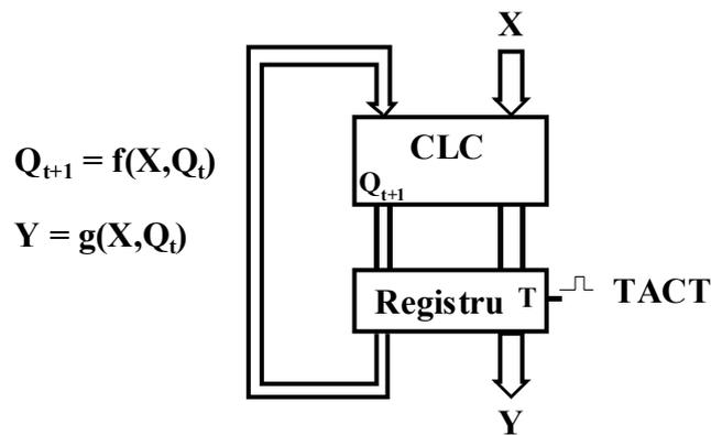
**Figure 1. Sequential logic system**
