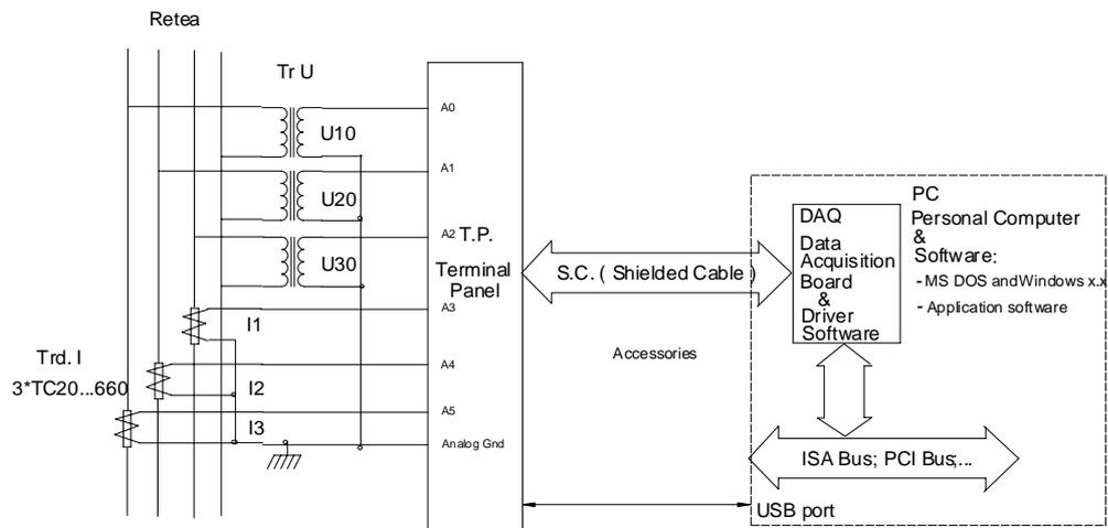
Figure 1. Basis scheme the of the quality analyzer
