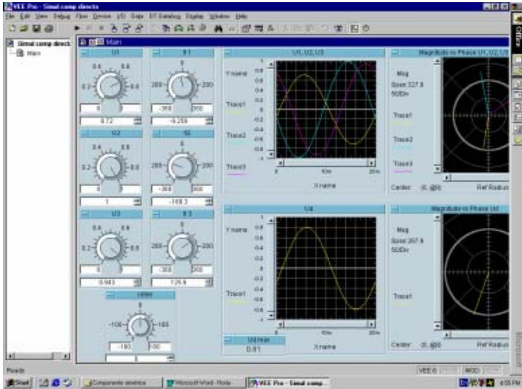
Figure 5. The simulator interface of direct components
