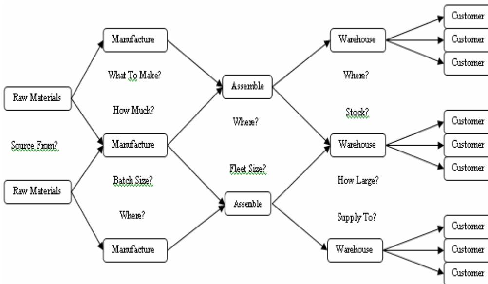
Logistics systems can be arbitrarily complex and difficult to understand. Some of the characteristics needed for modelling are listed in the table below:
