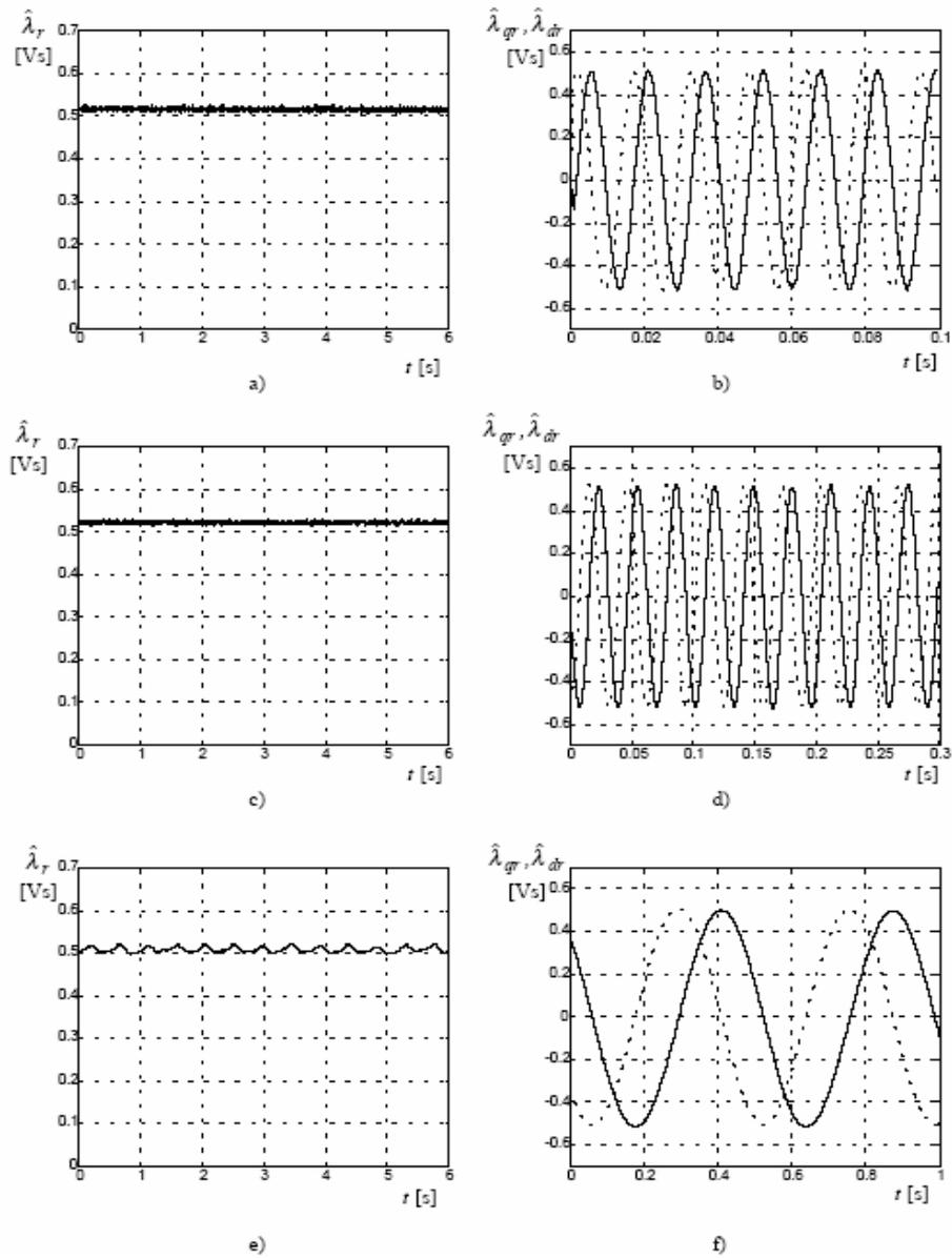
Fig. 1. Estimated rotor flux magnitude and components on stator 'q' and 'd' (dotted) axis. Luenberger observer, in off-line operation, 0.2 ms sampling time - experimental results.
