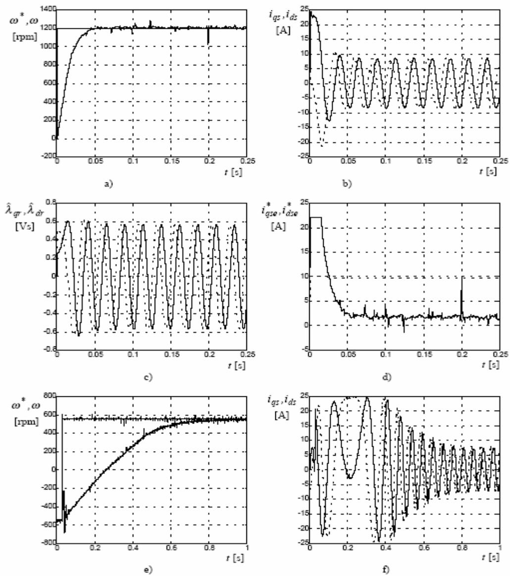
Fig.2. Starting and reversal process for a DFOC system based on a Luenberger flux observer. The sampling time is 0.2 ms - experimental results.
