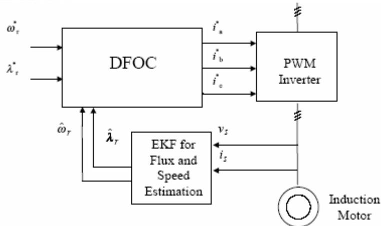
Fig. 4. Structure of a sensorless DFOC, based on EKF speed estimation method.
