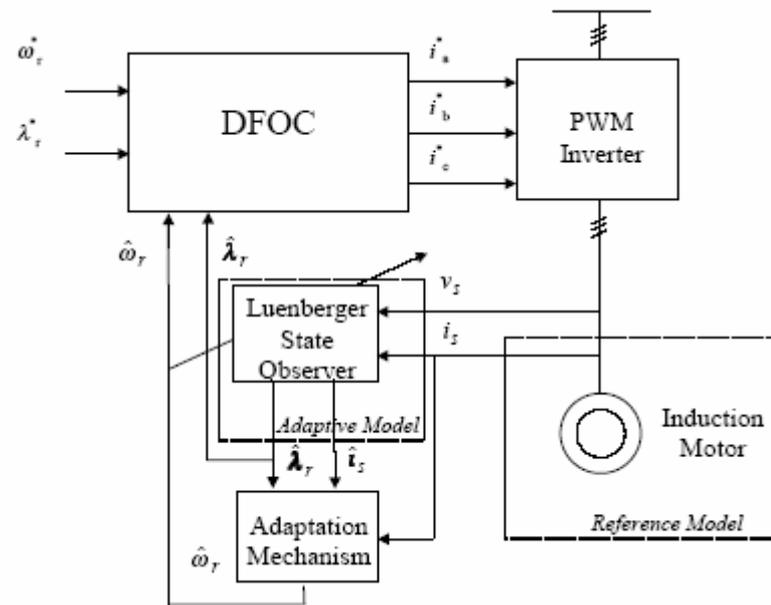
Fig.3. Structure of a sensorless DFOC, based on ELO speed estimation method.
