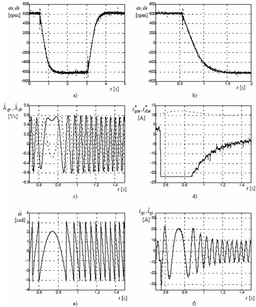
Fig. 6. Simulation results for an EKF sensorless drive.
