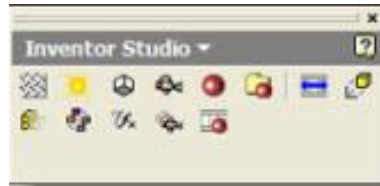
Figure 1: The Autodesk Inventor Studio control panel includes tools for rendering and animation effects
